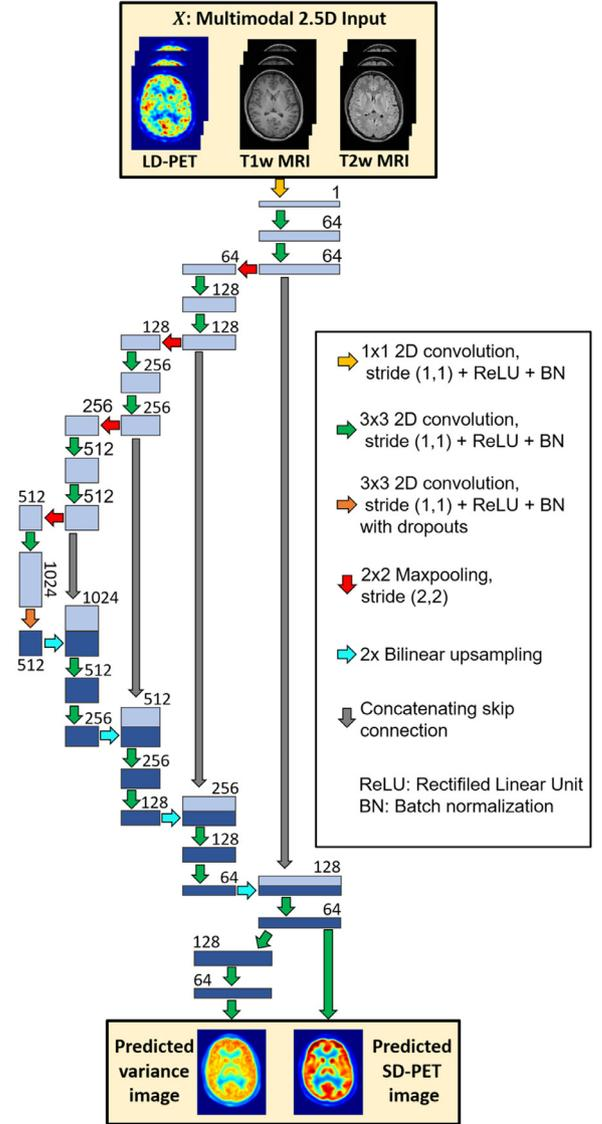
Fig. 2. suDNN Architectural Details. The numbers adjoining the blue boxes indicate the number of feature maps obtained at that stage. (For interpretation of the references to colour in this figure legend, the reader is referred to the web version of this article.)
